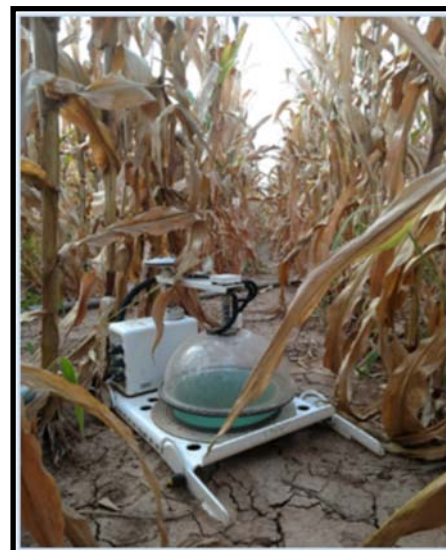
Automated soil chamber system that measured soil CO 2 flux during the growing season of corn and sorghum in 2019.
